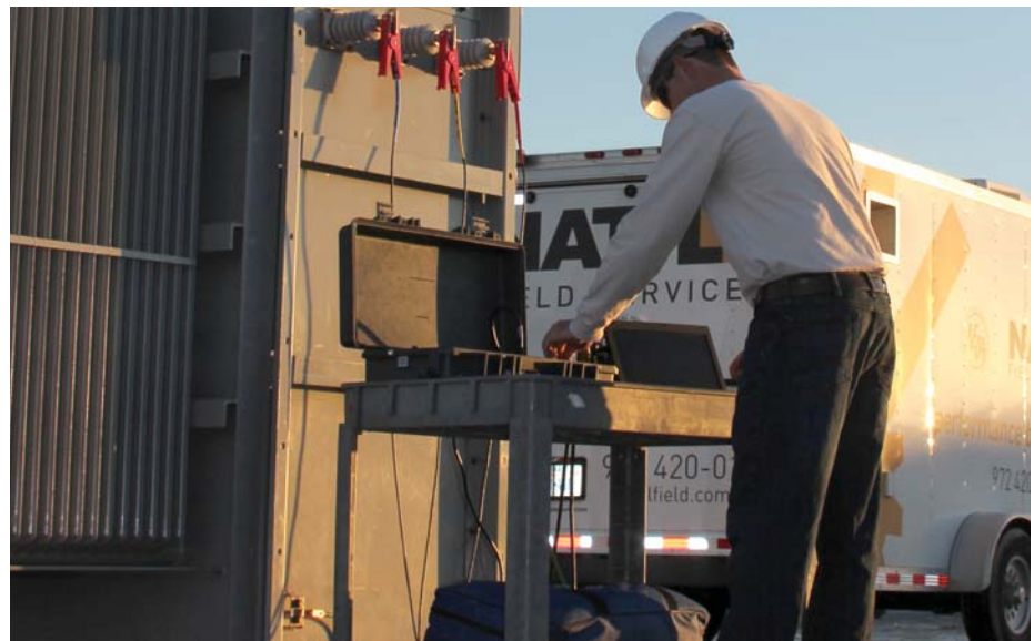
A NETA-certified ETT performs a power factor test on a de-energized 3,750kVA transformer.
